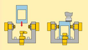
Swing cylinders used in conjunction with work supports and other Enerpac components to positively hold the workpieces during machining operations.
