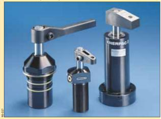
Enerpac swing cylinders allow unobstructed part fixturing and placement. The plunger rod and the attached clamp arm, rotate 90 degrees in either a clockwise or counter clockwise direction, then travel down an additional distance to clamp against the fixtured part. Upon release of clamping pressure, the clamp arm rotates back 90 degrees in the opposite direction to allow for part removal and new part placement.
