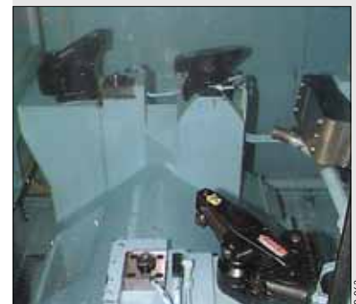
View of a machining fixture with ASC-30 clamping cylinders.
