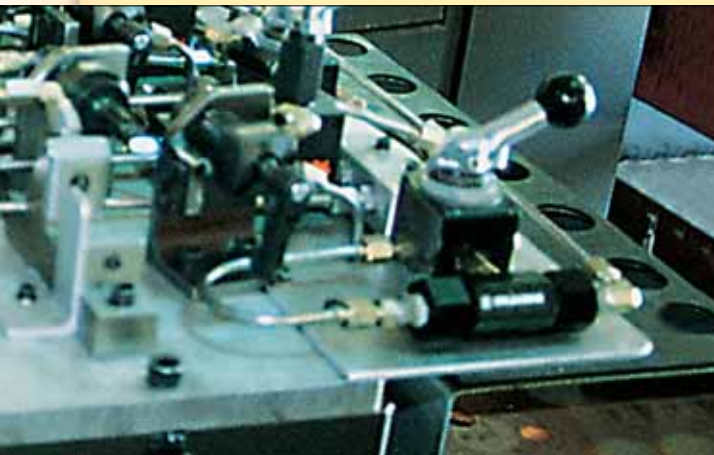
■ V-17 Safety check valve installed on a fixture.
