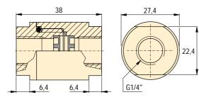
20 micron filter provides the longest service life
